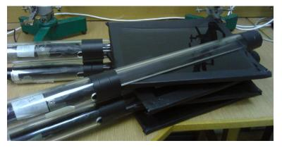
In order to plateau a counter, you need to set up the detector with 2 counters, one on top of the other. One will be the counter which you want to plateau, which we will call Counter 1, and the other will be your reference counter, which we will call Counter 2.
