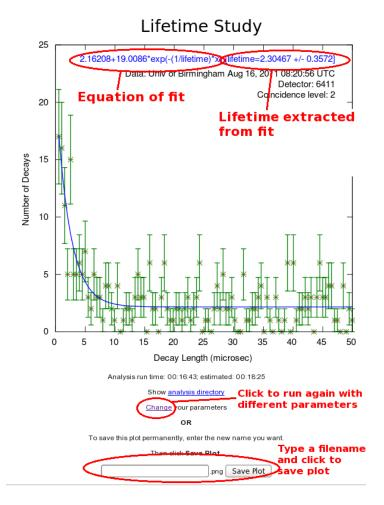
You should obtain a plot similar to the one above. The green points are your plotted data and the blue line is the exponential decay line which has been fitted. The formula for this fit is written at the top of the plot, and tells you the best fit for the lifetime of the muon. This is given in microseconds ( $\mu$ s, which is 1 millionth of a second.
