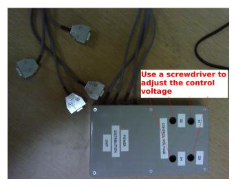
You can test the control voltage on each counter by plugging a digital multimeter (DMM) into the PDU across the 0V (black) and control voltage (white) plugs. Each counter has a separate plug for its control voltage. The control voltage can then be changed by turning the corresponding variable resistor in the PDU.
