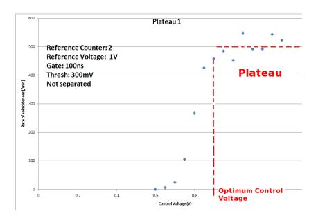
Your plot should look similar to the one above. There should be very few counts below a certain point, and when the control voltage is large enough that the signals are above the threshold, then the counts per minute should increase. The counts per minute should level off when all the cosmic rays are being detected. This levelling off is called the plateau. The operating voltage should be set to the voltage just above where the plateau begins.
