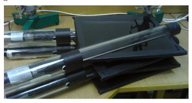
In order to plateau a counter, you need to set up the detector with 2 counters, one on top of the other. One will be the counter which you want to plateau, which we will call Counter 1, and the other will be your reference counter, which we will call Counter 2.
