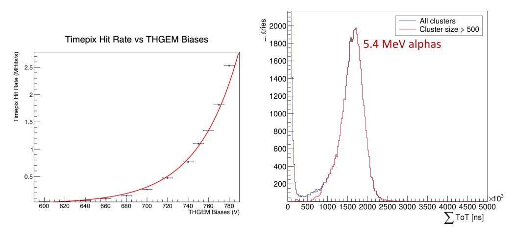
Camera pixel hit rate vs applied THGEM bias
