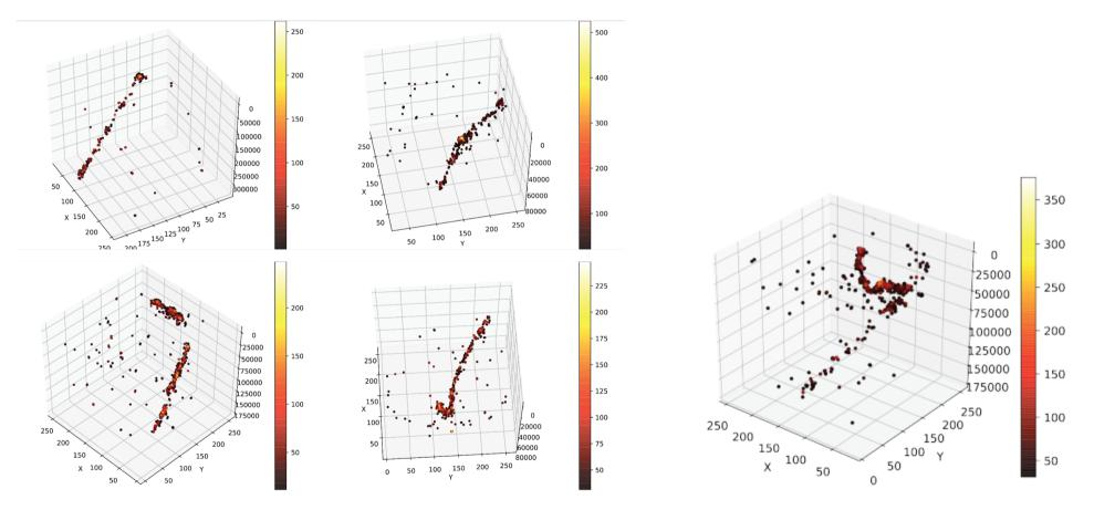
First demonstration of 3D optical readout of a TPC using a single photon sensitive Timepix3 based camera (<u>https://arxiv.org/abs/1810.09955</u>)
