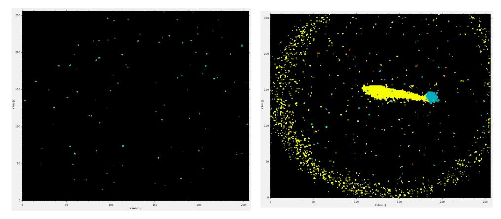
First demonstration of 3D optical readout of a TPC using a single photon sensitive Timepix3 based camera (<u>https://arxiv.org/abs/1810.09955</u>)
