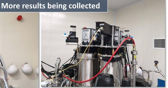
• One EMCCD replaced with TPX3Cam
