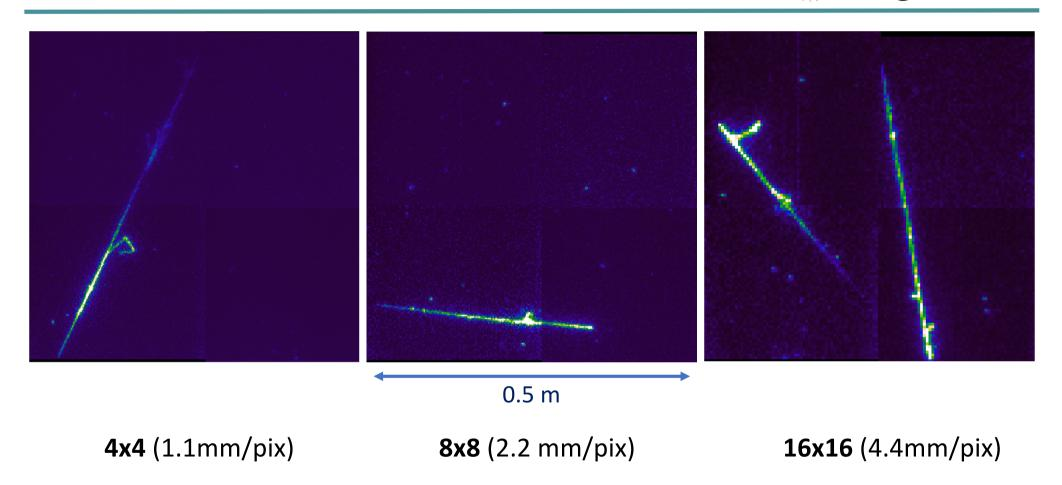
16x16 binning = 4.4mm/pixel, for kton scale LArTPC detectors resolution will be limited by electron diffusion (~4.2mm over 12m drift).
