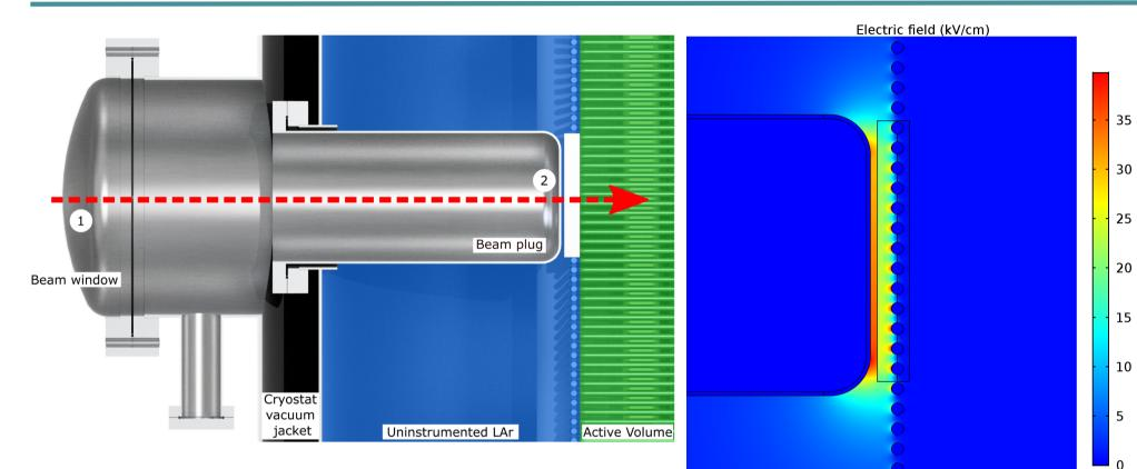
Beam transport through the ARIADNE beam window, plug and UHMWPE element.
