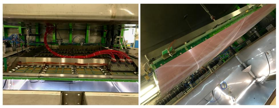
The Charge Readout Planes (CRP)
