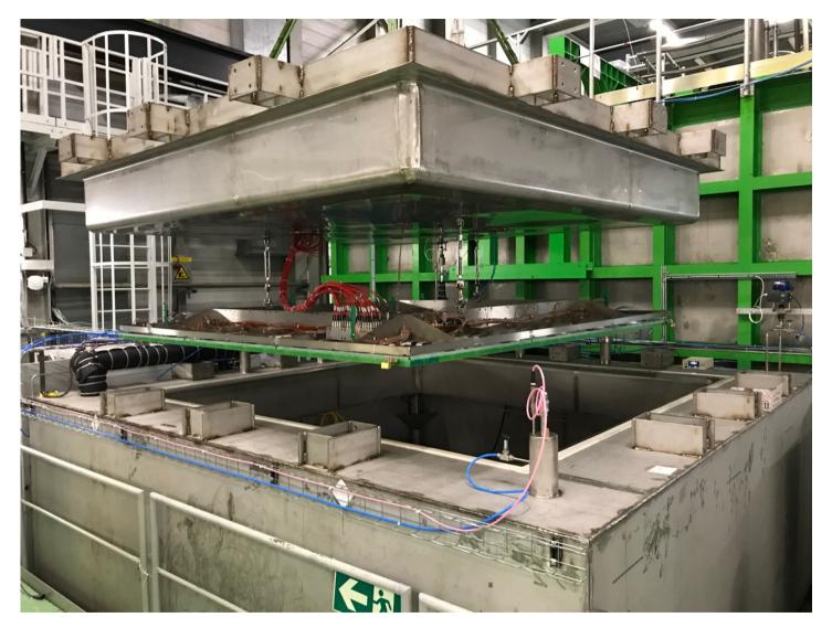
The cryo-vessel used to test the protoDUNE THGEMs will be modified and a full optical TPC will be instrumented
