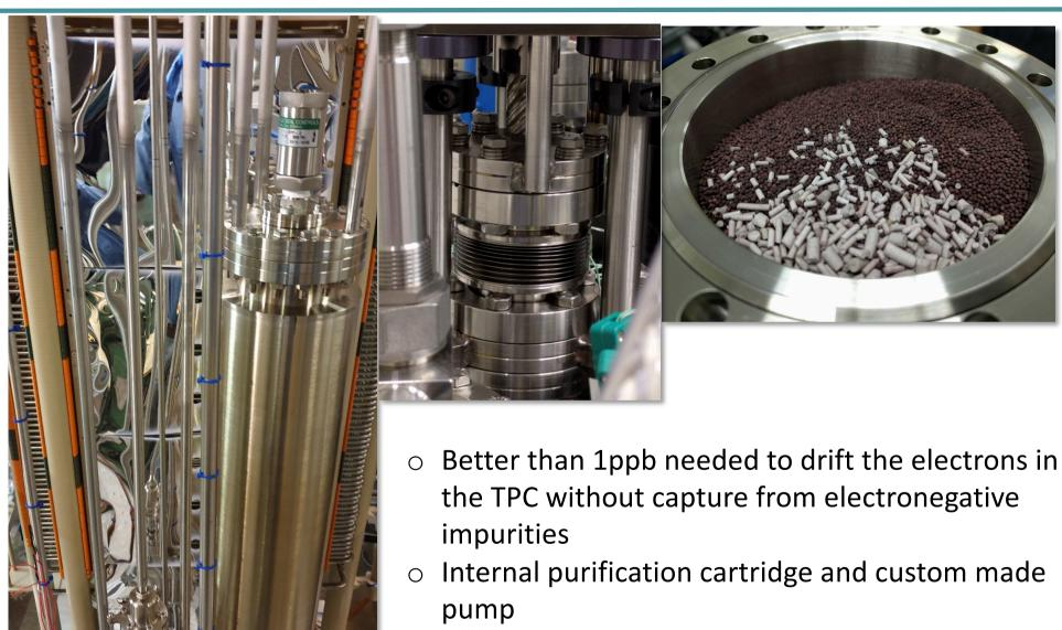
A Molecular sieves for water and Cu-0226 S for oxygen
