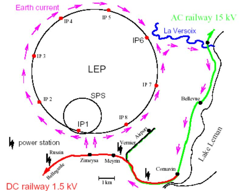
Compelling correlation between current on track, on beam pipe & noise in magnets.
