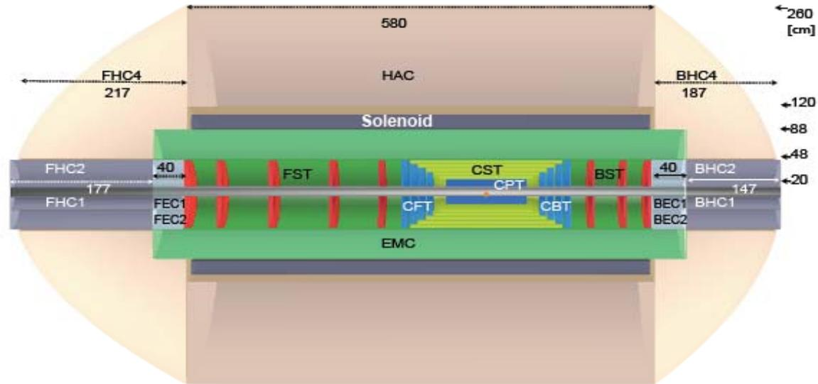
Figure 13.3: An  $rz$  cross section and dimensions of the main detector (muon detector not shown) for the Ring-Ring detector version (no dipoles) extending the polar angle acceptance to about  $1^\circ$  in forward and  $179^\circ$  in backward direction.
