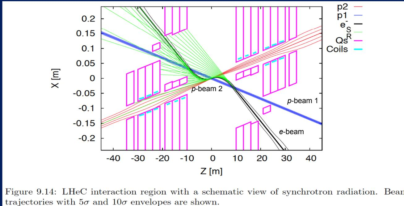
Figure 9.14: LHeC interaction region with a schematic view of synchrotron radiation. Beam trajectories with  $5\sigma$  and  $10\sigma$  envelopes are shown.
