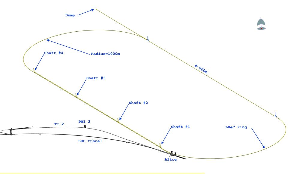
60 GeV Energy Recovery Linac = 2 shafts Or 140 GeV pulsed Machine = 4 shafts
