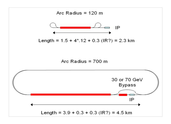
60 GeV 31 MV/m, pulsed two passes 60 GeV 13 MV/m CW ERL 4 passes 140 GeV
