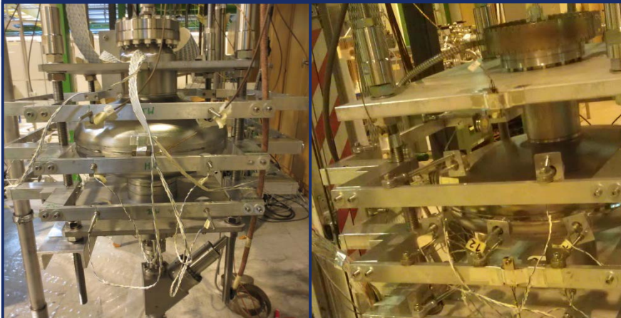
Quench localization via second sound on SPL cavities
