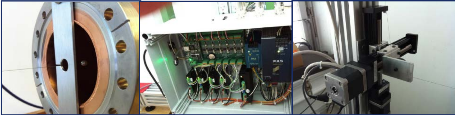
Bead-pull measurement setup for field mapping
