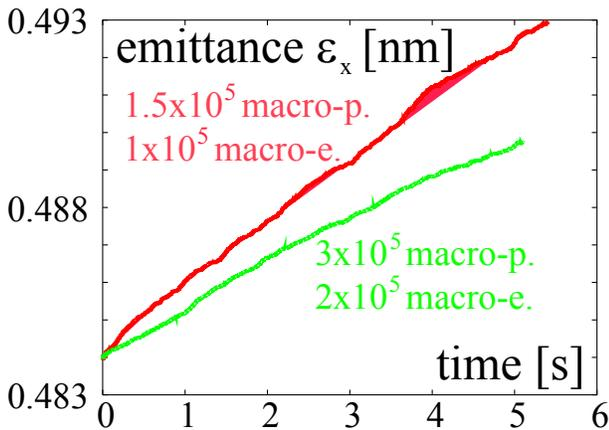
Figure 6: Simulation of proton-beam emittance growth due to collision with 75-GeV electron beam at  $\xi \approx 0.005$  on every 111th turn, for two different numbers of macroparticles. A modified version of the program HEADTAIL was employed.
