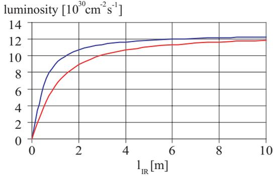
Figure 3: Luminosity in the LHC-CLIC QCD Explorer versus the length of the interaction region. The luminosity is shown for  $\beta^* = 0.25$  m (top curve, blue) and for  $\beta^* = 0.5$  m (bottom curve, red).
